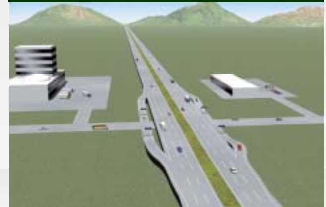
Smart Interchange (diamond-shape)
