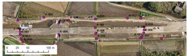
Fig.3 GCP Placement in Target Area
