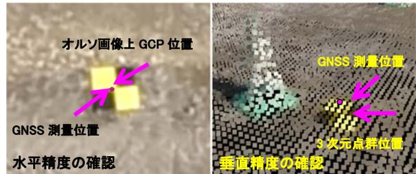
Fig.11 Accuracy verification at Checking Points and GCP
