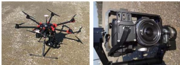
Fig.2 UAV (S900) and Camera (NEX-7)
