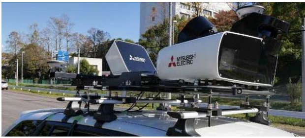
図-1 MMS-AT220(低密度MMS)
