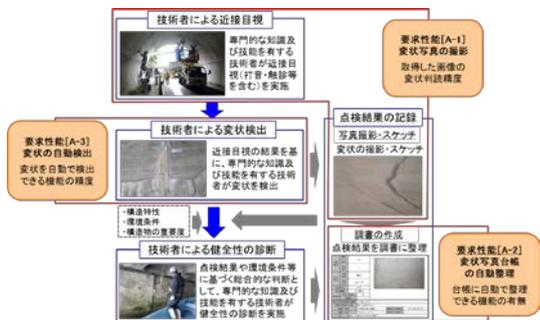
Fig. 5 The relationship between work-flow of the current tunnel inspection method and the requirement
