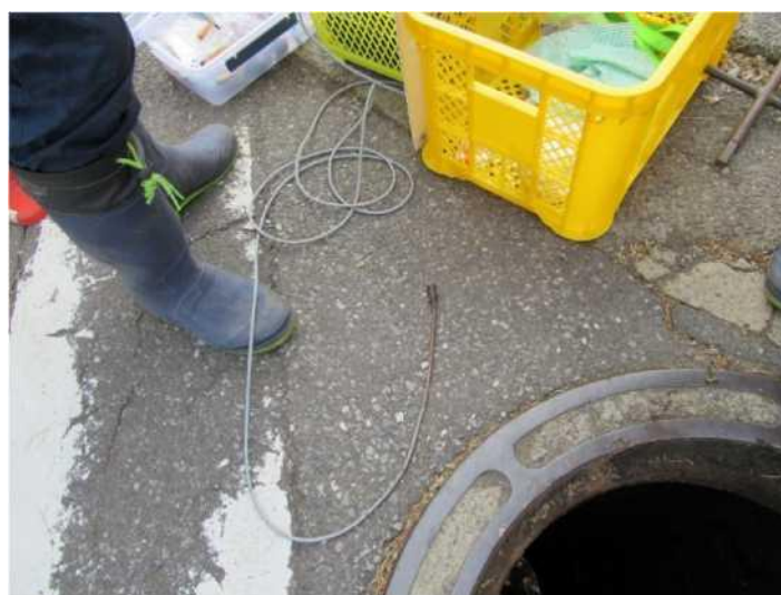
Figure 2-12 Situation of submerged external microphone (Jonan Treatment District, Tsukuba City)
