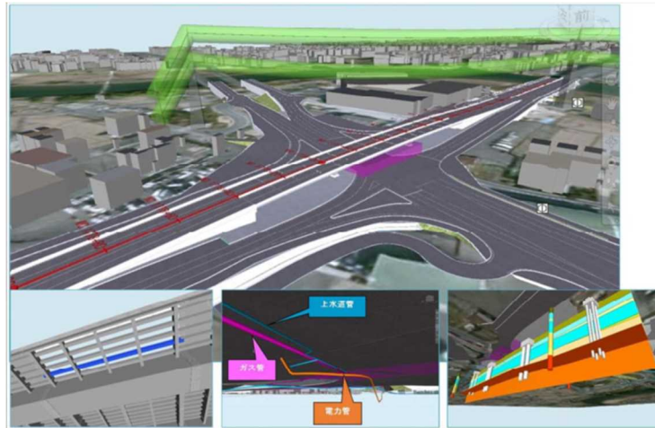
図-3-9 BIM/CIM を用いた占用物等確認
