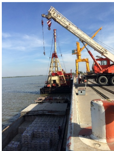
Figure 4-11 Small scale ship crane and crawler crane
