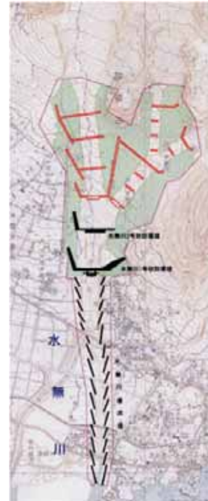
Fig. 2: Improvement plan of the sediment control facilities on the Mizunashi River of Unzen and Fugendake
