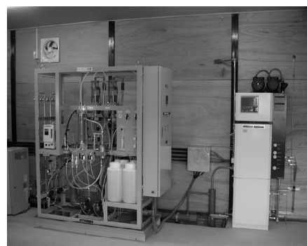
Photo-2 Odor-Causing Compound Detection Equipment (VOC Monitoring System)
