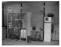
Photo-2 Odor-Causing Compound Detection Equipment (VOC Monitoring System)
