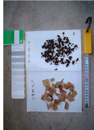
Steam-exploded broadleaf tree chips prepared under pressure of 2MPa for 15 minutes.
