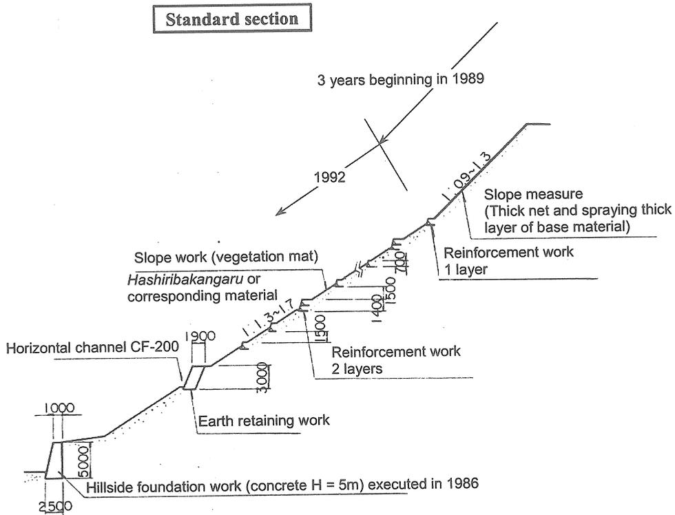
(15) The topography is accurately assessed to perform dependable treatment of the surface water and the underground flow on the slope.
