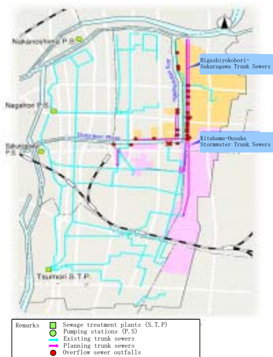
Fig. 4: Stormwater Storage Pipe along Dotonbori River for CSO Control
