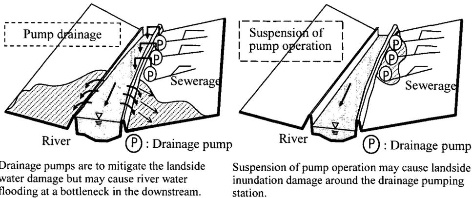
Figure 2 Image of Inundation Caused by Drainage Pumps
