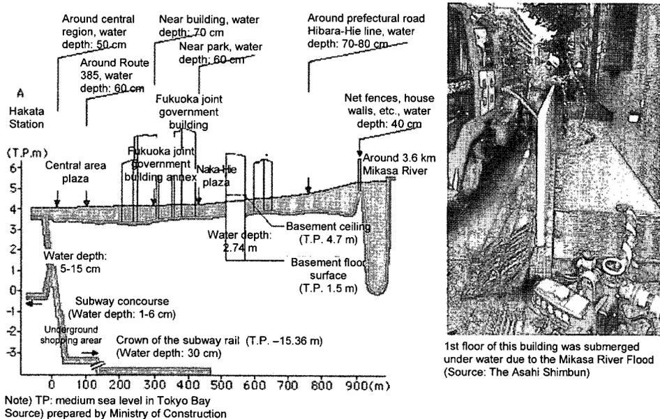
Figure 1 Cross-Sectional View of Inundation in Fukuoka Flood
