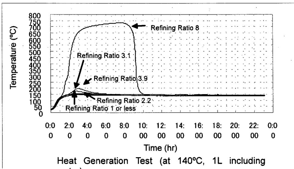
Figure 9 Refining Ratio and Self- Exothermic Characteristic
