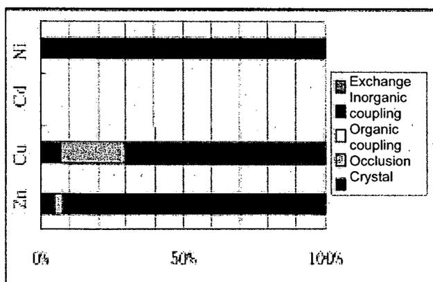
Note: Since more than 90% of heavy metals are retained in the crystal or occlusion state, the possibility of elution under the natural environment is very low.
