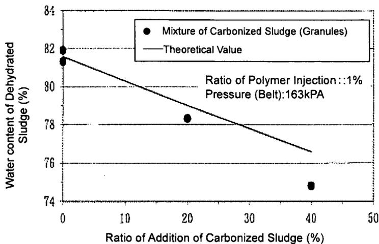
Note: By adding carbonized products, sludge cakes having a lower moisture percentage than theoretical value by 0.5 to 2% were produced. The carbonized product is presumed to have coagulation effect.
