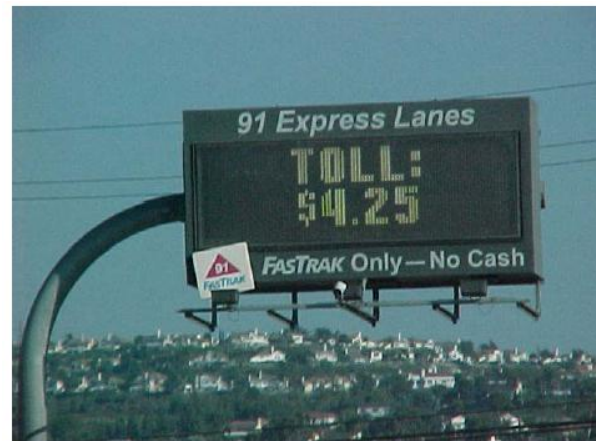
Figure 9. Dynamic Message Price Sign Used on SR 91 in California.
