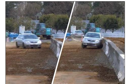
Photo: Testing collision between actual car and protective fence
