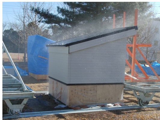
Photo Status of strong wind seepage test on outer wall and roof
