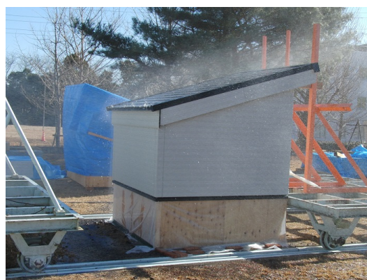
Photo Status of strong wind seepage test on outer wall and roof
