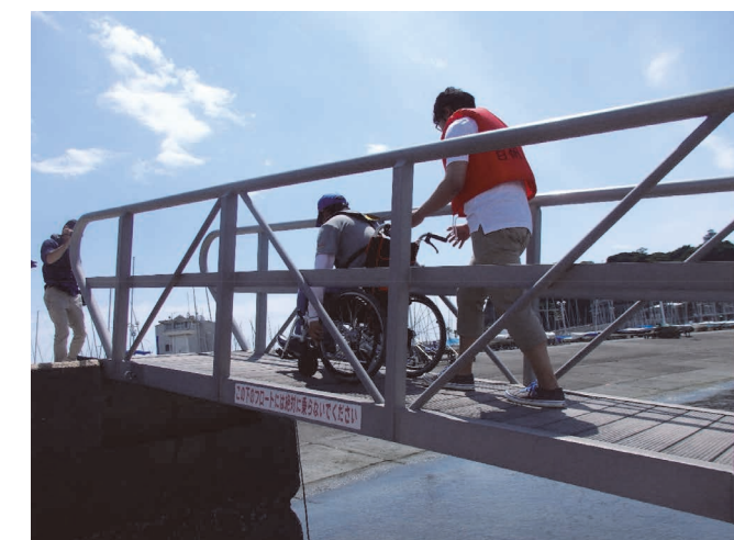
Photo Wheelchair during the proving test of a connecting bridge
