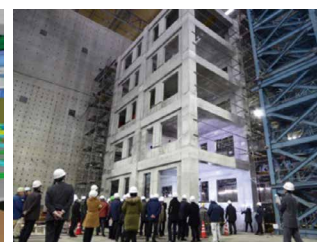
Photo: Loading test of a full-size 5-floor RC building using walls to reduce damage during earthquakes.
