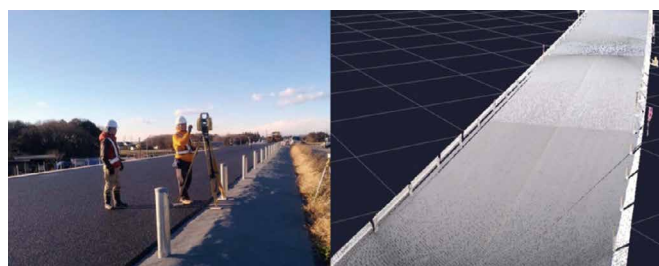
Figure. Completed work measurements using a laser scanner (left) and acquired point group data (right)
