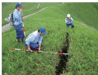
Photo 1. Surveying cracking caused by the earthquake
