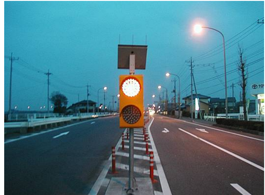
Self-lighting obstruction warning light
