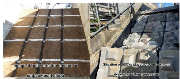
Photo-3 Experiment image having gully erosion at embankment slope
