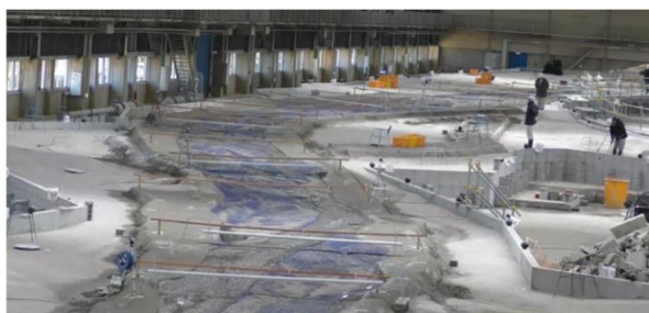
Photo: Hydraulic model experiment to understand polarization process of river channel
