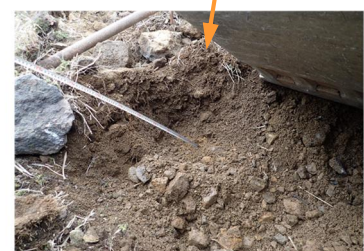
Survey for the backside of deformed openings for re-flapped materials (No deformation suspected of slipping on the dam's body)
