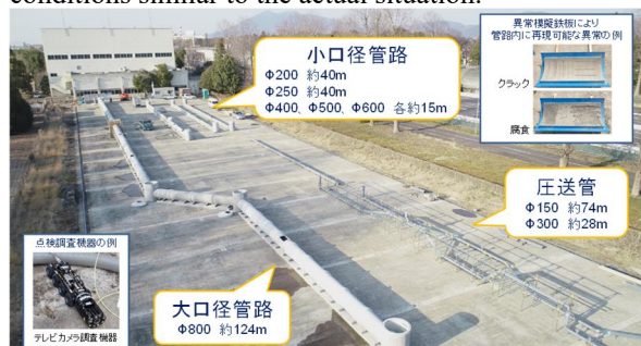
Figure-1 Bird's eye view of sewerage pipeline simulation facilities
