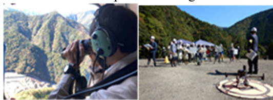
Photo-1 Measurement of a natural dam (Left: measurement from helicopter, right: measurement by UAV)
