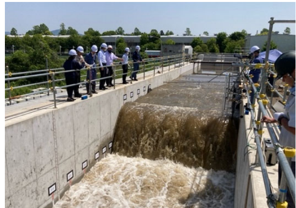
Photo-3 Actual-size overtopping experiment using large-scale experimental facility
