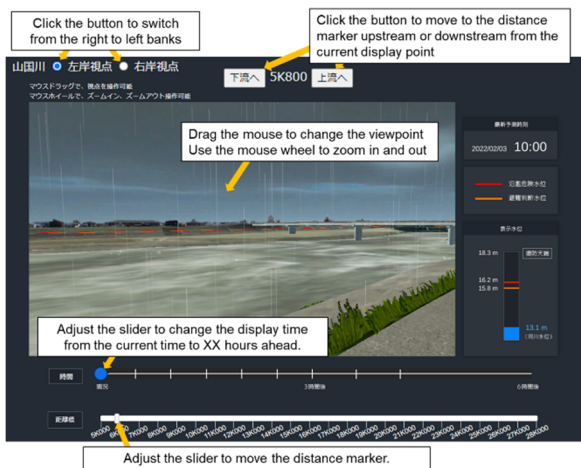
Figure 2. Operational screen for VR display we developed
