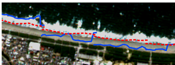
Figure 2. Difference of extraction results by shoreline extraction method Top: Bottom: Example of wrongly extracted detached breakwaters, Bottom: Example of wrongly extracted wave breaking zone and coastal forest (blue solid line: edge extraction, red dashed line: deep learning)
