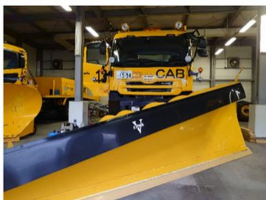
Photo 1: Example of airport snow removal vehicle (snowplow)
