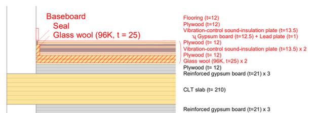
**Fig. 2: Example of measured floor section specifications<sup>3)</sup>**
