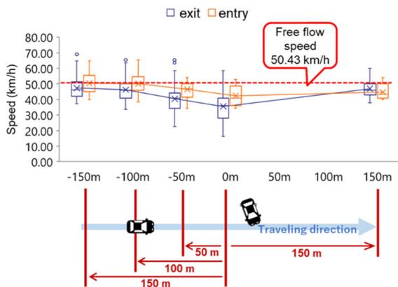
Fig. 2. Change in speed in vehicles directly behind entering and exiting vehicles
