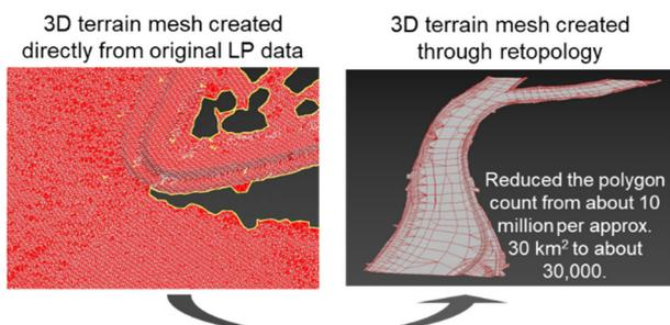
Figure 1. Retopology (reattaching a surface according to shape)
