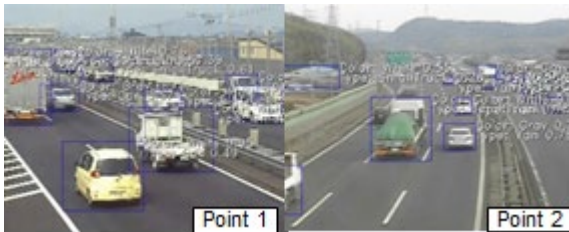
Photo 1 Example of AI traffic counting technology
