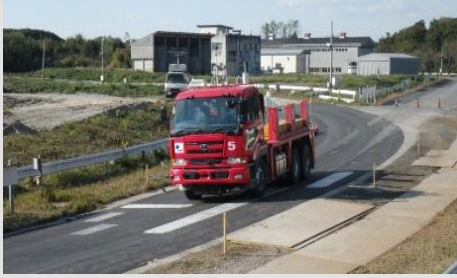
Photo : Accelerated loading tests for pavement and underground cables
