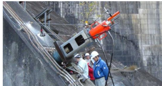
Figure 2. Lift-off Test Conducted in Trial Inspection
