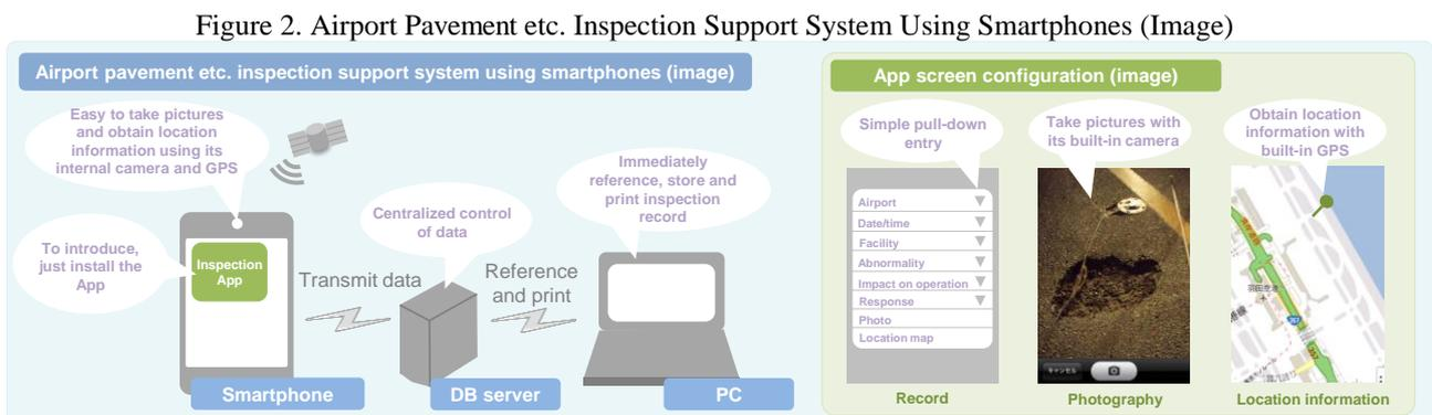
Figure 2. Airport Pavement etc. Inspection Support System Using Smartphones (Image)
