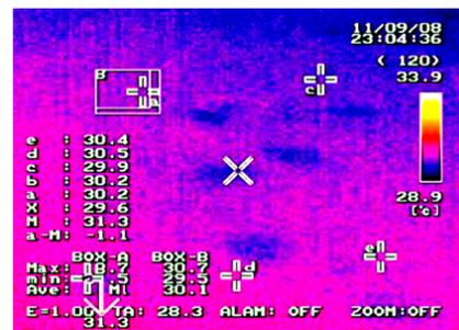
Figure 1. Infrared image (center blue circles indicate low temperature part due to de-bonding)
