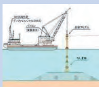
As-built shape measurement by using construction history data (left: mechanical leveling (foundation works), right: grab dredging ship (floor digging works))
