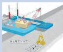
As-built shape measurement by using construction history data (left: mechanical leveling (foundation works), right: grab dredging ship (floor digging works))
