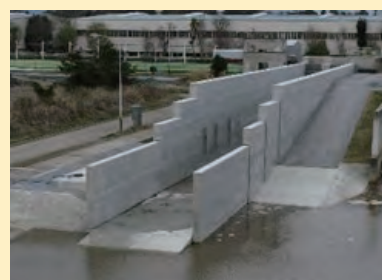
Construction of an experimental channel to enable the overflow experiments necessary to study the development of tenacious river levees.
