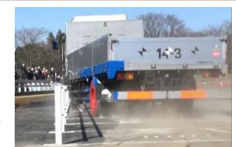
View of full-scale vehicle collision test of guard fences for residential roads
