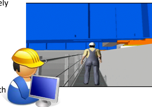
Walkthrough simulation (confirmation of “ease of inspection”, etc. when designing)
