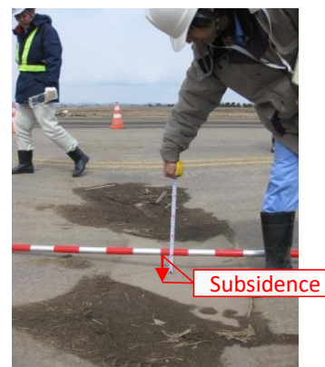
Local subsidence of taxiway (asphalt pavement) by liquefaction
