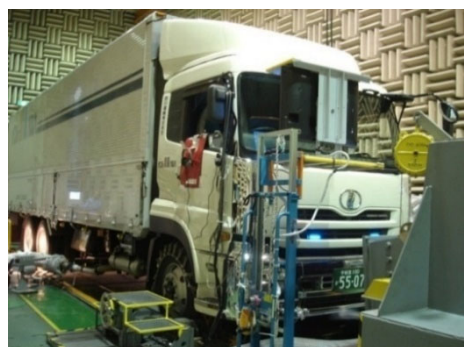
Photo-1 Emission gas measurement simulating actual driving
