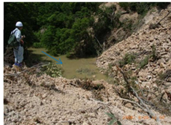
Figure-2 Field survey of river channel blockage (natural dam) by the Landslide Research Department (Iwate-Miyagi Nairiku Earthquake in 2008)
