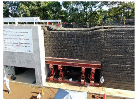
Figure 3: Test to confirm resistance of pavement structure with geogrid to deformation caused by ground deformation
