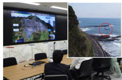
Photo 9: Experiment of information acquisition by an auto-navigating UAV
