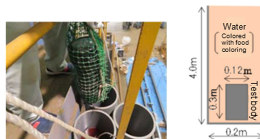
Figure 10 Water resistance verification test of cable sheath repaired by the proposed method (Condition in which a cable specimen is put into water with food coloring)
