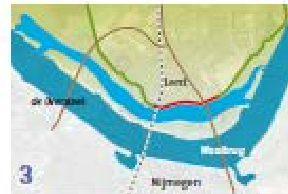
3 An ancillary channel is to be dug in order to give the river more room. This will create an elongated island.
