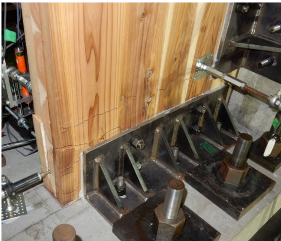
(e) CLT 袖壁の端部の亀裂 ( R=1/50 )
