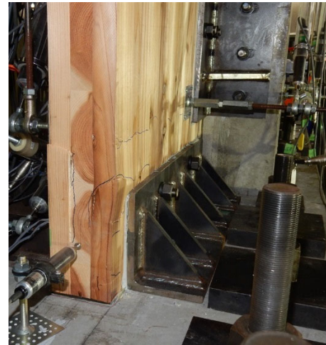
(e) CLT 袖壁の端部の亀裂 ( R=1/50 )
