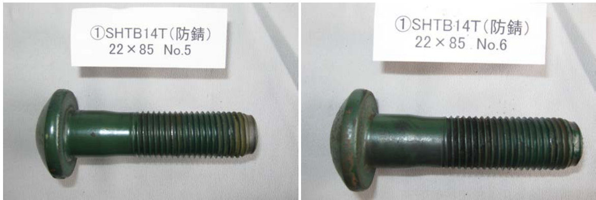
(a) ①S14T (防錆処理)
