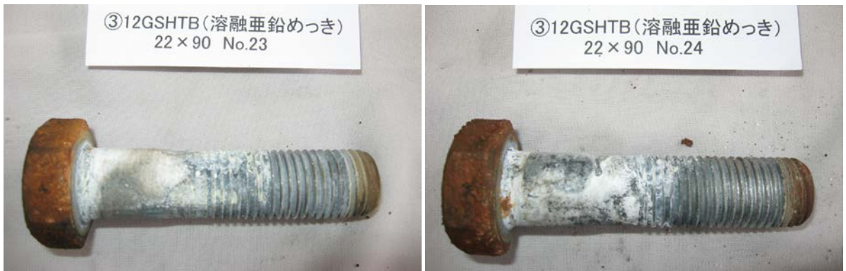
(c) ③F12T (溶融亜鉛めっき処理)
