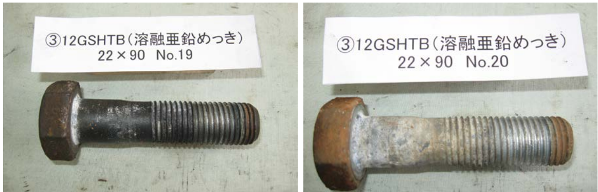
(c) ③F12T (溶融亜鉛めっき処理)
