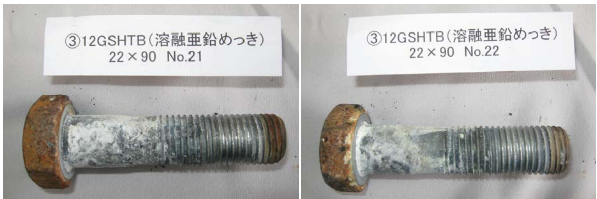
(c) ③F12T (溶融亜鉛めっき処理)
