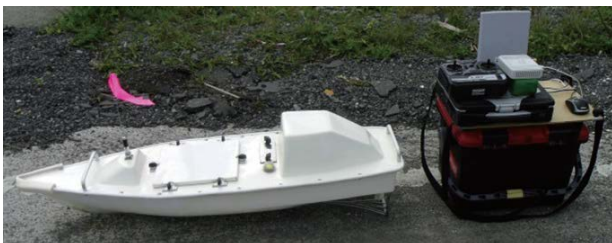
図-4.22 UMV (Unmanned Maritime Vehicle) 51)
