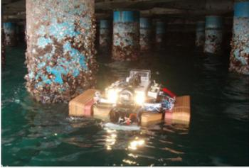
栈橋係船岸の床版下面の点検用ROV
