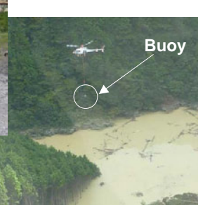
Throwing PWRI water level observation buoy
