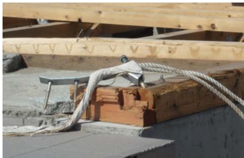
Photo.7.4-5. Failed hold down fastener.
